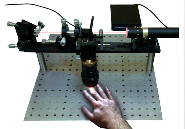
Experimental setup: nail bed was illuminated by He-Ne laser ( $\lambda=633$  nm) via beam expander and collimating mirror and resulting speckle images were captured via CMOS camera by PC.
