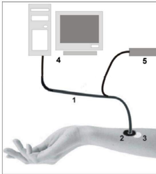
Fig. 2. Scheme of experimental setup for measurement of blood perfusion: 1 – optical cable which has two optical fibres; 2 – the double sided adhesive disc to hold the position of the optical cable; 3 – the place of glucose injection (the light circle is the swelling of the skin); 4 – computer; 5 – diode laser
