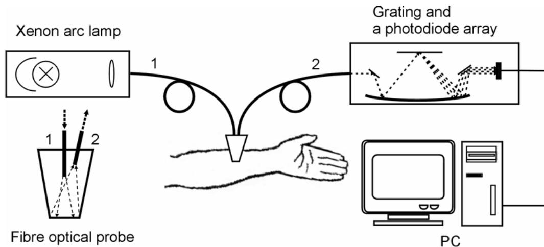
Fig. 1. Experimental set-up for measurements of the reflectance spectra:
