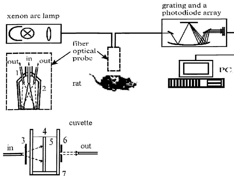
**Figure 1.** Experimental setup for measurements of the collimated transmittance and the reflectance spectra: 1 – optical fiber; 2 – aluminum jacket; 3 – neutral filters; 4 – rat skin sample; 5 – osmotically active solution (40%-glucose solution); 6 - the 0.5 mm – diaphragm; 7 – cuvette.
