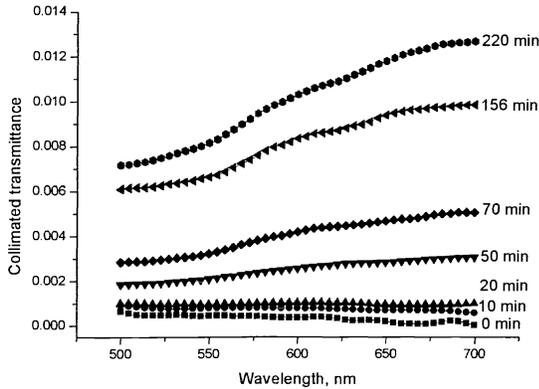
**Figure 3.** Typical collimated transmittance spectra of the rat skin sample (sample 1) measured concurrently with administration of the 40%-glucose solution at different time intervals.
