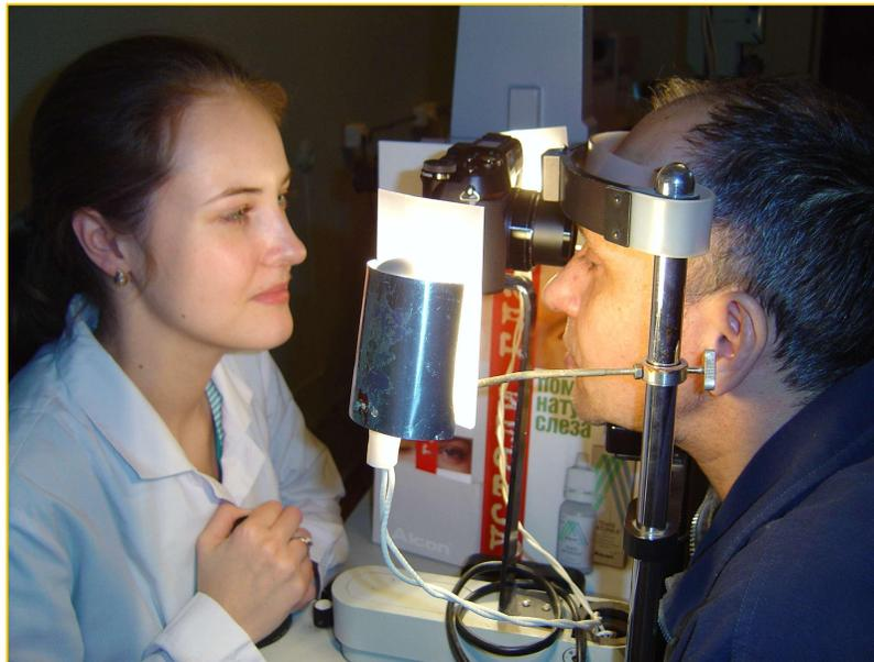
Figure 7: Experimental setup for *in vivo* registration of digital images of human irises
