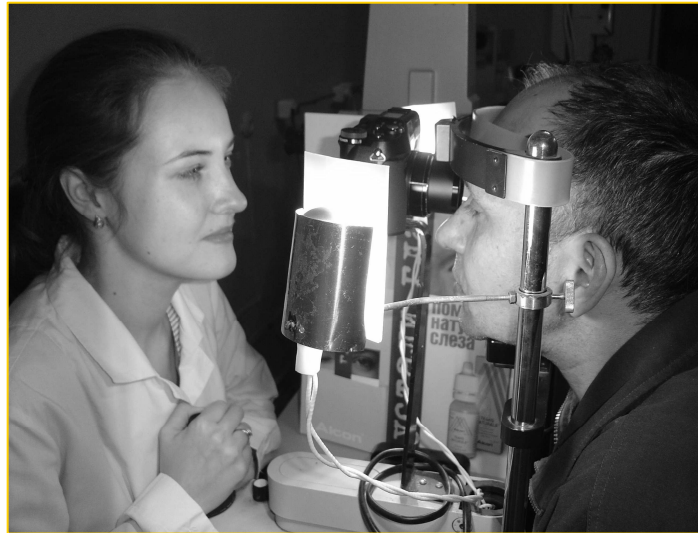
Fig. 7. Experimental setup for in vivo registration of digital images of human irises
