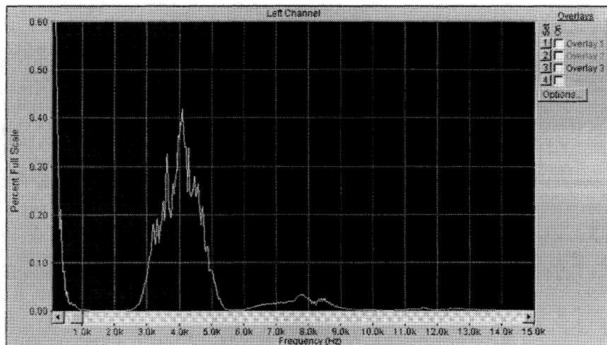
Fig.2: Doppler frequency shift power spectrum obtained with rotating disk.
