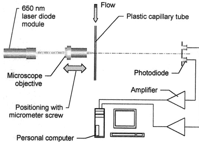
Fig.3: Speckle-interferometric instrument for monitoring of capillary bio-flow.
