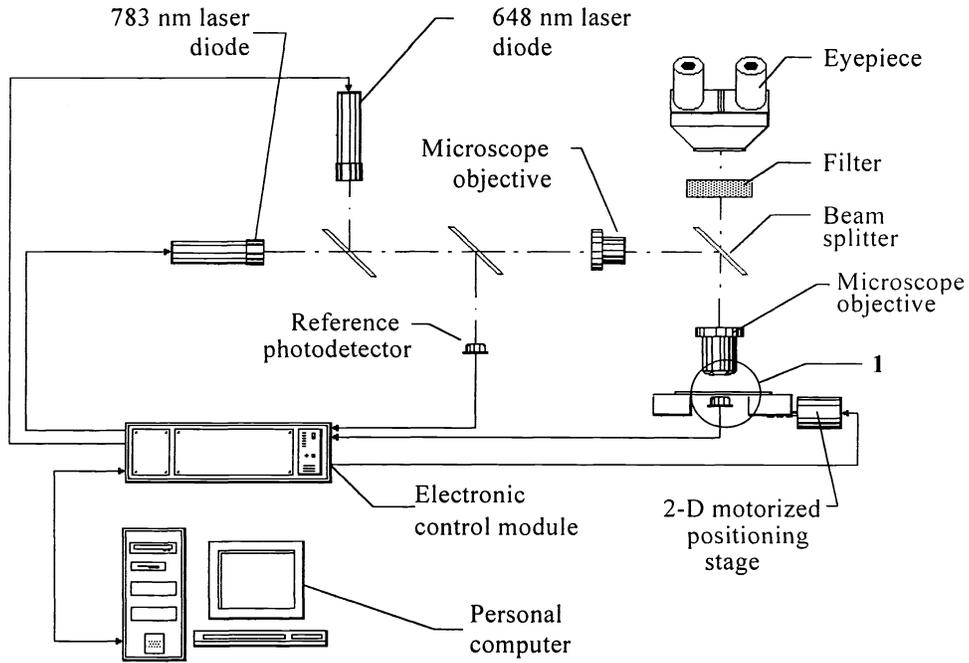
Fig. 6: Optical scheme of two-wavelength laser scanning microphotometer.
