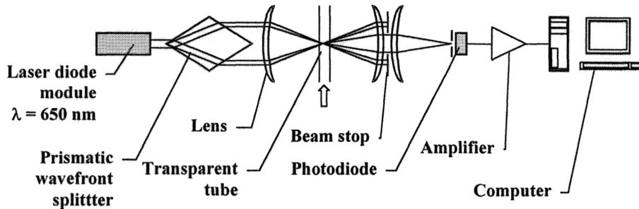
Fig. 1: Optical scheme of laser Doppler velocimeter
