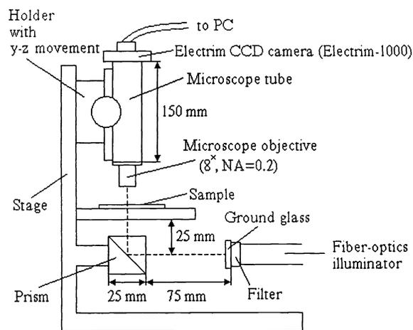
Fig. 13: Optical scheme of spatial-resolved microspectrophotometer for tissue optical properties and geometry studies: CCD tester
