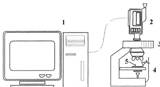
Fig. 8: Video-microscopic system for spatial digital color analysis of biological objects: 1 – PC, 2 – CCD-camera, 3 – light microscope, 4 – light sources for transmittance or reflectance measurements, 5 – biological object.
