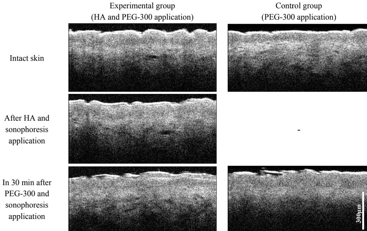
Figure 1. The typical OCT scans of the skin areas from experimental and control groups at the different stages of experiment
