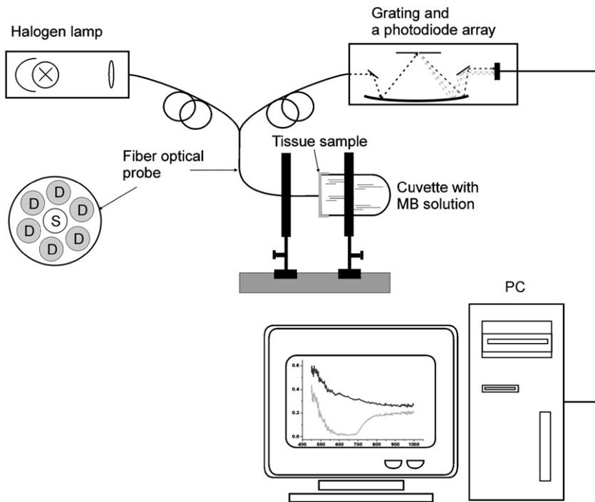
**Fig. 2.** Experimental setup for measurements of the spectral characteristics of skin. S is the source of irradiation, D are detectors.
