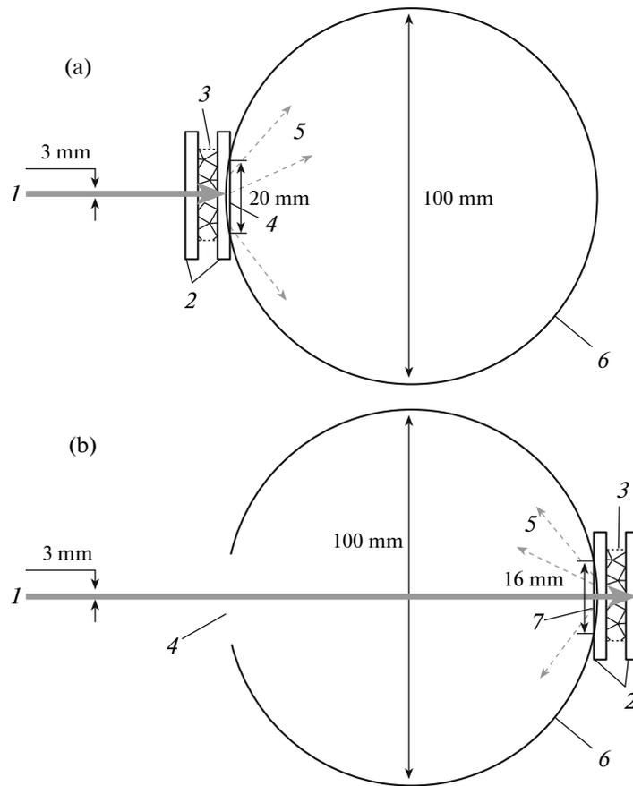
**Fig. 1.** Geometry of measurements of (a) total transmittance and (b) diffuse reflectance of a sample of skin: (1) incident beam (with a diameter of 3 mm), (2) slides, (3) skin sample, (4) entrance hole, (5) transmitted (or diffusely reflected) light, (6) integrating sphere, and (7) exit hole.
