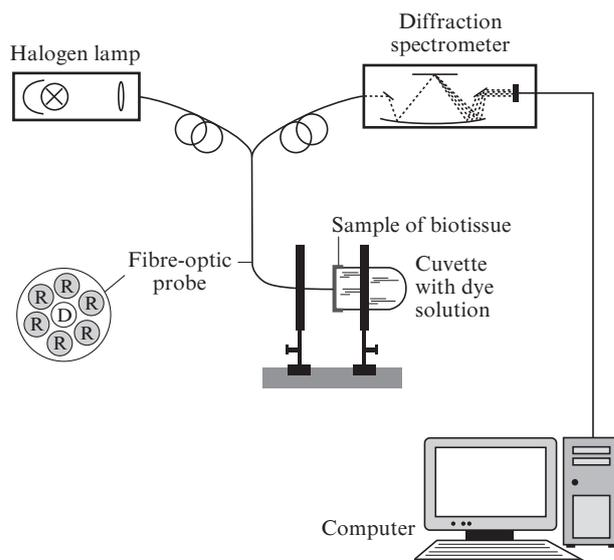
Figure 1. Scheme of the experimental setup (R – receiving fibre, D – delivering fibre).
