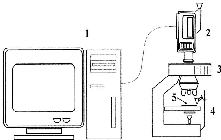
Fig. 2: The scheme of microscopic digital imaging system: 1 – PC, 2 – color video camera, 3 – light microscope, 4 - illuminating system provided as transmission as reflection modes of illumination, 5 – investigated object (skin sample).
