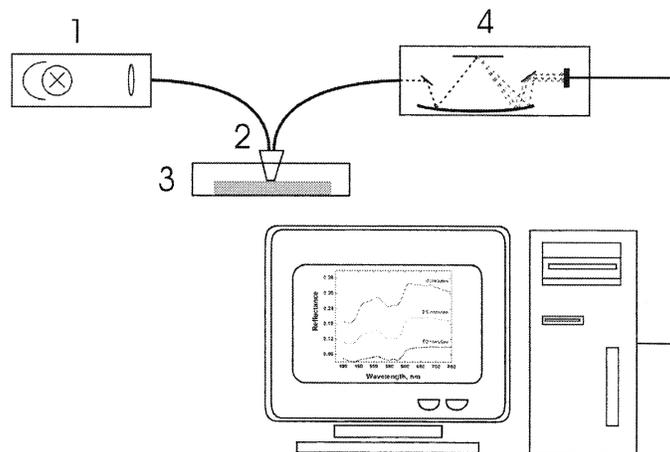
Figure 2: The geometry of the measurements in reflectance mode with the spectrophotometer LESA-5: 1 - galogen lamp; 2 - fiber-optical probe; 3 - cuvette with a bone sample; 4 - grating and photodiode array.
