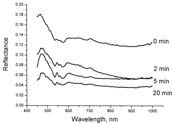
Figure 5: The reflectance spectra of the bone sample measured concurrently with administration of propylene glycol at different time intervals.
