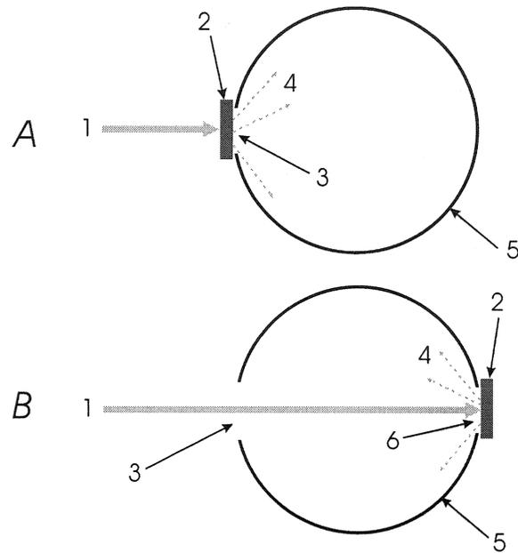
Figure 1: The geometry of the measurements in A) transmittance mode, B) reflectance mode: 1 - the incident beam (diameter 3 mm); 2 - the bone sample; 3 - the entrance port (square 20×20 mm); 4 - the transmitted (or diffuse reflected) radiation; 5 - the integrating sphere (inner diameter is 100 mm); 6 - the exit port (diameter 16 mm).
