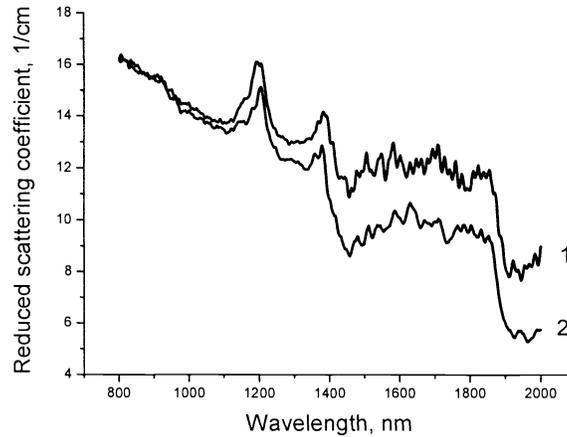
Figure 4: The reduced scattering spectra of bone sample measured before (1) and after administration of glycerol (2) during an hour.
