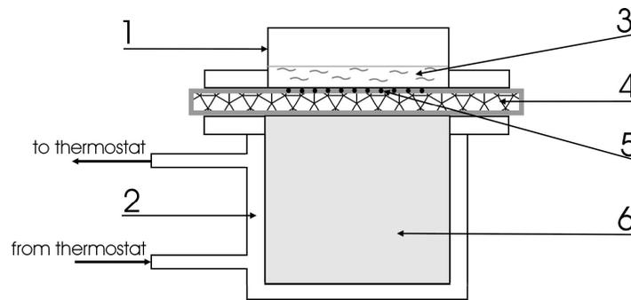
Fig. 1. Scheme of cuvette for the study of the refractive index change: 1 – upper reservoir of the cuvette; 2 – temperature-controlled lower reservoir of the cuvette; 3 – studied agent, in which refractive index is measured (water or glycerol solution), the volume of the liquid is 2 ml; 4 – skin sample; 5 – epidermal layer with/without LIDs; 6 – glycerol or saline, the volume of the liquid is 20 ml.
