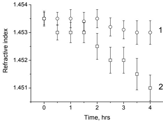
Fig. 5. The dynamics of glycerol refractive index during skin dehydration through epidermis. 1 – the sample with non-damaged epidermis and 2 – the sample with damaged epidermis.
