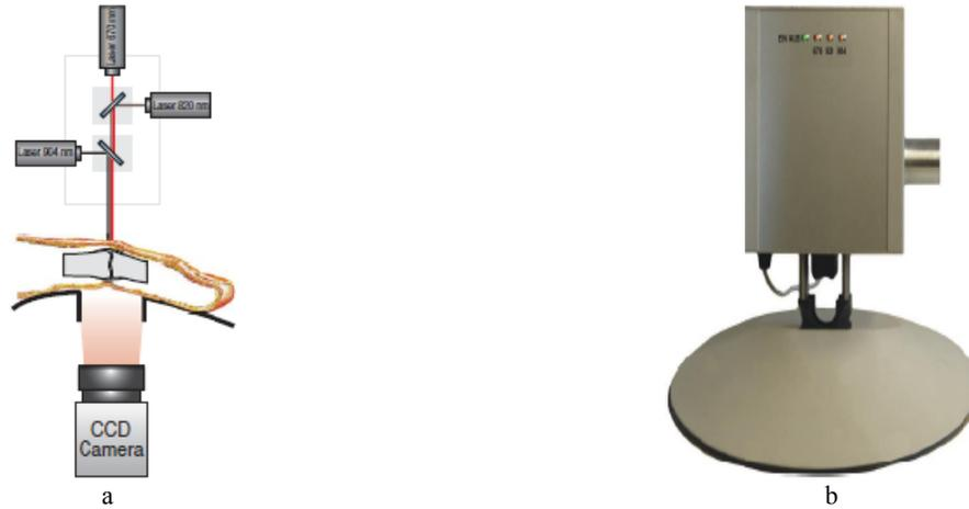
Figure 1. The exterior of the experiment (a) and the transillumination system with 3 laser diodes (b).
