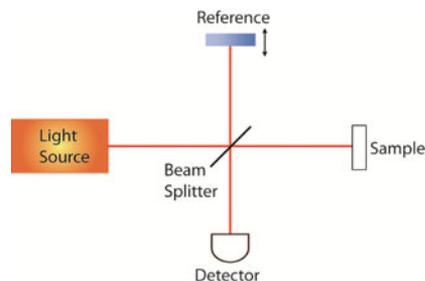
Fig. 1. Simplified diagram of a low-coherence interferometer.
