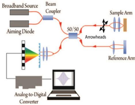
Fig. 3. Spectral-domain OCT.
