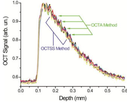
Fig. 5. OCT signals recorded at different times to indicate region and depths for both OCTSS and OCTA analysis methods.
