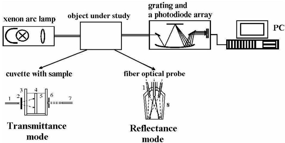
Fig 2 Experimental setup for measurements of collimated transmittance and reflectance spectra from tissue: 1 – optical irradiating fiber; 2 – neutral filters; 3 – cuvette; 4 – tissue sample; 5 – osmotically active immersion agent; 6 – the 0.5 mm – diaphragm; 7 – optical receiving fiber; 8 – aluminum holder.
