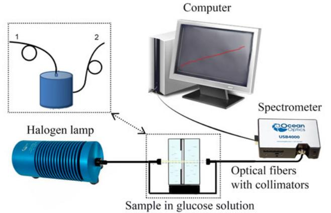
Fig. 1. The scheme of the experimental setup for *ex vivo* measurement of collimated transmittance spectra of skin samples immersed in the aqueous 40%-glucose solution. In the inset it is shown the integrating sphere for *in vivo* measurement of diffuse reflectance spectra of skin after injection of the aqueous 40%-glucose solution. 1 is the irradiating fiber, 2 is the collecting fiber.
