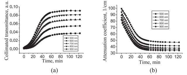
Fig. 6. Typical kinetic curves for collimated transmittance (a) and reconstructed corresponding attenuation coefficient (b) of *ex vivo* skin sample during its immersion in 40%-glucose solution measured for different wavelengths.
