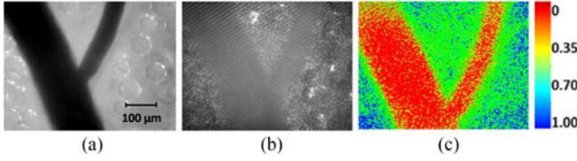
Fig. 3. The image of the vessel (diameter  $280 \mu\text{m}$ ) obtained by a digital microscopy (a), speckle image in coherent light (632.8 nm) (B&W) (b) and calculated distribution of laser speckle contrast (1-0) (colored). Scale corresponds to  $100 \mu\text{m}$ .
