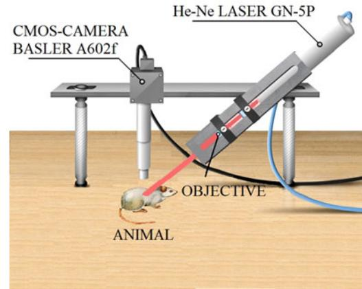
Fig. 2. The scheme of experimental setup for measurement of blood microcirculation in rat hypodermis.
