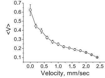
Fig. 5. Phantom studies: the experimental calibration curve: relationship between speckle contrast and velocity of particles.
