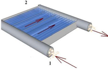
Fig. 4. Schematic representation of skin phantom: 1 is the suspension of particles (diameter  $\sim 7\text{--}9 \mu\text{m}$ ); 2 is the phantom with the surface area  $\sim 2 \times 2 \text{ cm}^2$ , number of channels (blood capillaries) of  $\sim 300$  and their diameters of  $\sim 180\text{--}200 \mu\text{m}$ .
